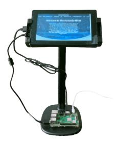
• The key hardware components of the kiosk device mode were the Raspberry Pi board and touch screen.
